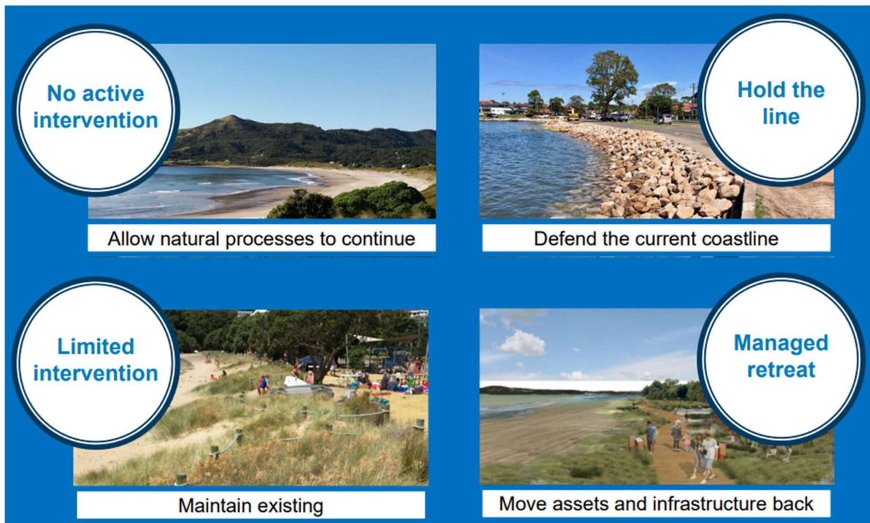
Figure 3-1: Adaptation strategies (sourced from Thames Coromandel District Council shoreline management planning consultation materials, see https://thames-coromandelcaps.ireport.royalhaskoningdhv.com/ )
